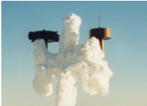
Figure 3. Ice free anemometer in severe icing conditions.
